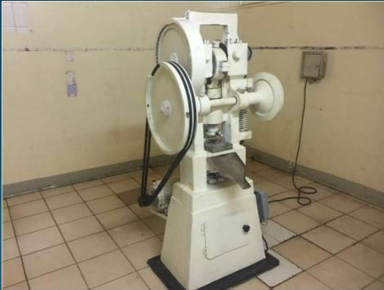
Rene Industries R&D tablet press that made the Artemisia tablets
